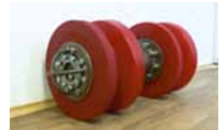
Cup-disk cleaning pig “VOSTOK-M4” with “VOSTOK-VR” installed in the front, prior to the trial.
